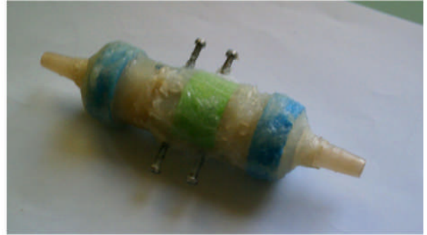
Fig. 4: The applicator. Tubing for the connection to the pump and to the collector can be easily fixed on both ends.
